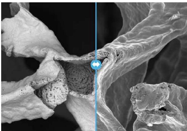
Figure 1 – Mixed mode, easy overlay of SE and BSE images
